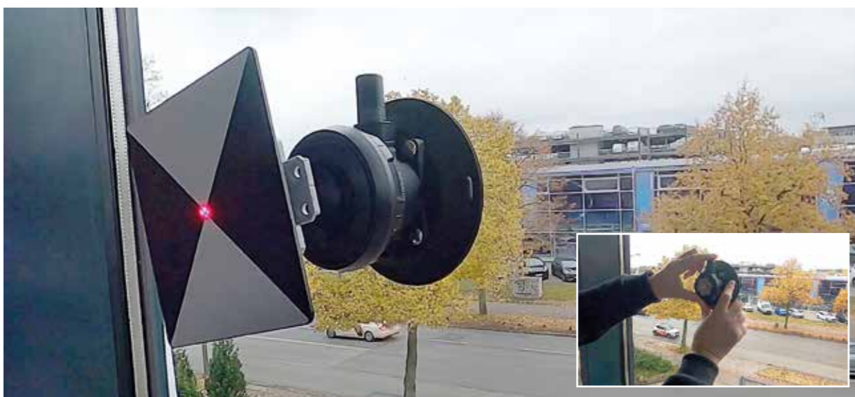
The image shows the use of the targets in combination with a NavVis instrument. Reference points for sockets RSFP-X90-30 to 36 and the suction cup RSSV-X90 are particularly very popular for indoor applications. You can find a related video on our YouTube channel.
