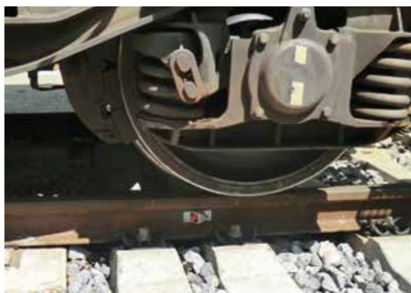
RSMP15 for surveying with robotic total station while under load
